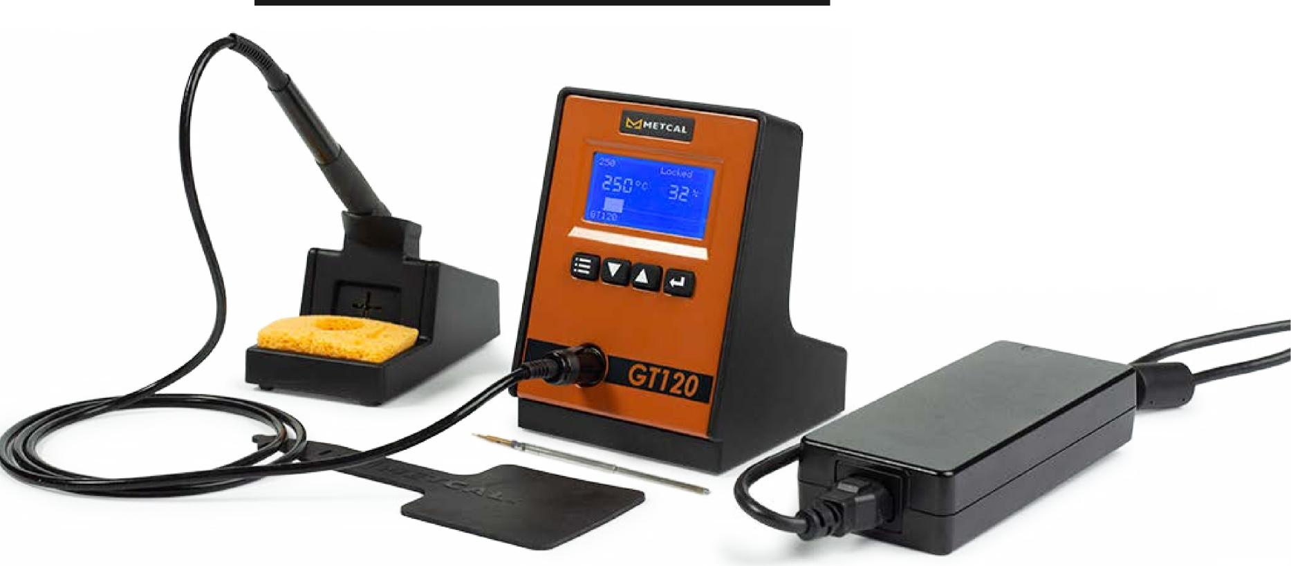
The GT120 Soldering System is an adjustable temperature station that uses inductive technology as the heating mechanism. The system includes a power station with adapter, hand-piece, heater cartridge, and workstand.
